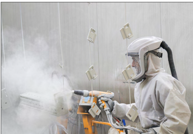
Powder coating with a spray gun
