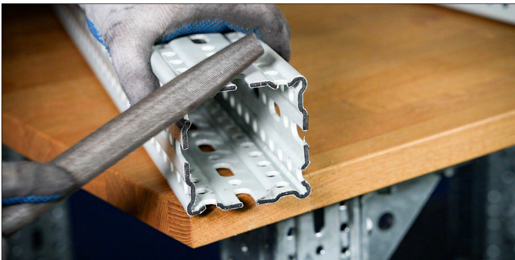
Treating cut edges with a hand file
